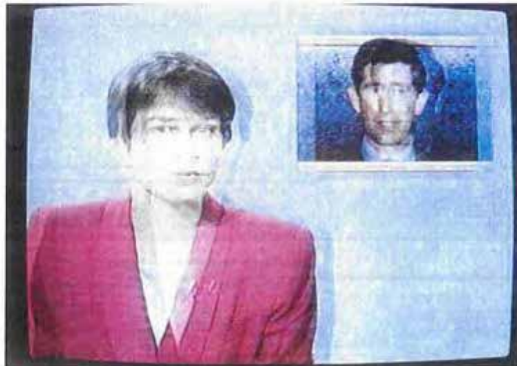
Photograph 1: An example of severe delayed image interference or 'ghosting' affecting analogue television reception.
